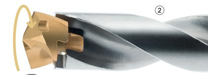
3 Fit the multi-key over the assembly notch. Turn the replaceable head. In this position, the required torque is increased, as the replaceable head is screwed in position.
