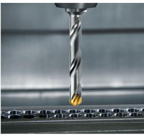
Material: 1.4571, V4A  $v_C = 70 \text{ m/min}$ ; f = 0.2 mm/rev
